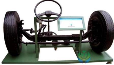
Power Steering System Complete Assembly (Model)
