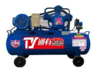
Rated power: 2.5kW, 3Hp and 230v motor Twin cylinder belt slow running pump. Tank capacity : 100 liter Start method : 13A Wheel : 4 Drive Belt Tank material : Steel Pressor: 8bar Pump (RPM ) : 1000 Motor speed (RPM ) : 2100 Air displacement : 300 liter per minute Included twin pressure gauges ,cut out switch .safety valve and pressure regulator. Productivity: 200 l/min Compete with all standard Accessories
