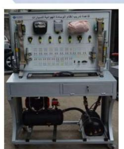
The experimental study of the functions managed by the air-bag control unit, as well as the modification of configuration.
